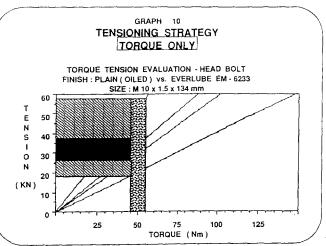
joint requirement. The minimum/maximum clamp load requirement is 22,500/42,500 lbs.
