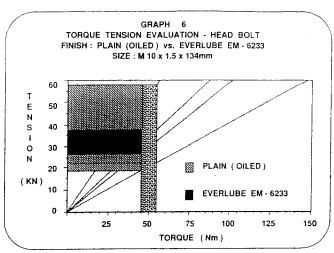
in this case Everlube EM-6233. This represents an 80% reduction in torque/tension variability. Graph 3 translates this reduction into a more meaningful result. We have arbitrarily selected a torque range of 25-35 ft-lb. By selecting ±3 sigma tension value at the min/max torque value for each finish, we are able to get a comparison of achievable tension ranges.
