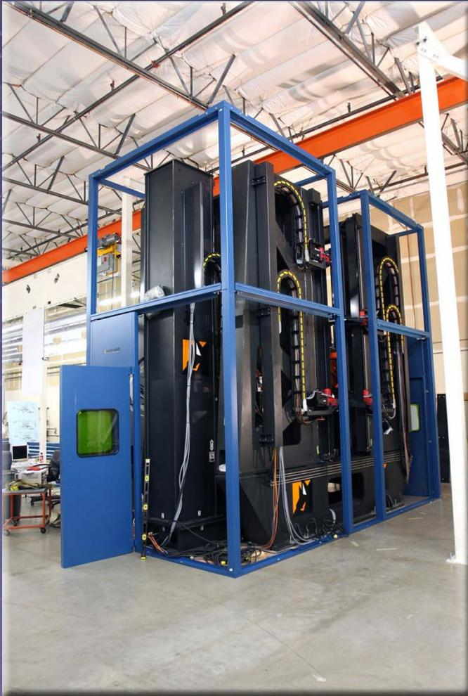
An overhead gantry transports wing skins through a fixed processing cell; the laser propagates ~150ft between the trailer and the cell.
