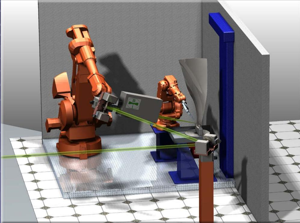
Mechanical design of the active beam delivery system
