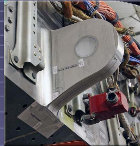
Optical metrology quickly and accurately adapts to variations in work piece location
