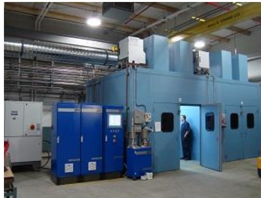
Booths with integrated robot and multi-process TS System
