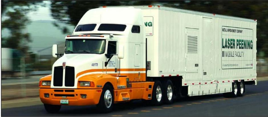
The Mobile Laser Peening Facility contains a fully equipped peening system that can be set up at field sites in less than one week, then dis-assembled and made ready for transport to another site in approximately two days.
