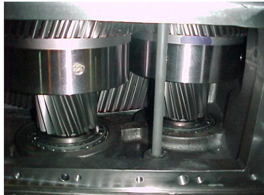
Figure 4: Heavy Duty Marine Transmission Transfer Gears.
